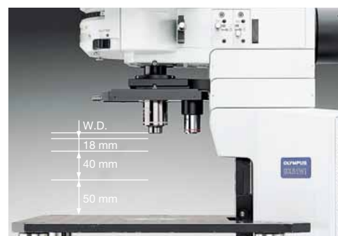
Detaching the condenser assembly and lowering the stage by 50 mm provides maximal clearance
